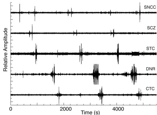
**Figure 2.** Horizontal component (east-west) of the seismic trace shown for a subset of stations (SNCC, SCZ, STC, DNR, and CTC). The traces indicate the changing character of the signal as a function of distance from the source. Waveforms are high pass filtered above 9 Hz.
