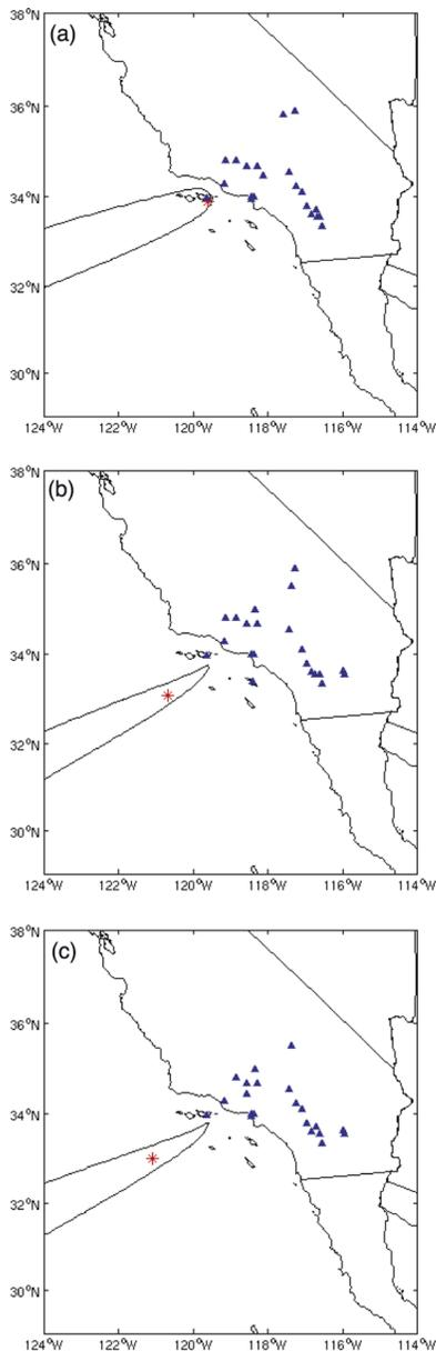
**Figure 4.** Best fit source locations for the 3 signals shown in Figure 1b on day 046 in 2003. The stars give the best fits for the available data. Each ellipse gives the 95% confidence interval, as explained in the text. Note that the fits are not well determined as all of the stations fall to the west of the source, but each signal shows a similar back azimuth.
